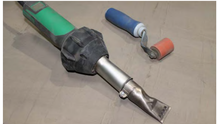
A Hand-held heat gun with 40mm slot nozzle & a 45mm seam roller
