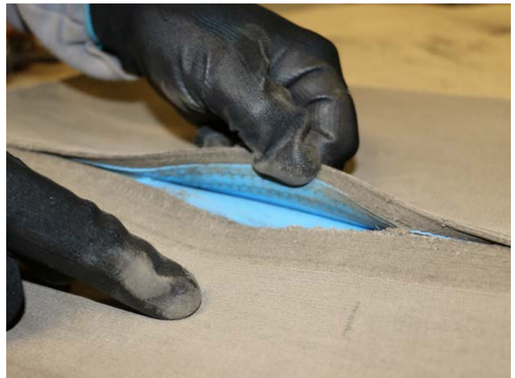
Weld Track C would need to be opened carefully to access Weld Track B
